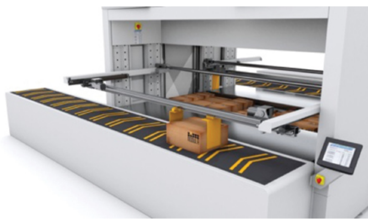
A secure delivery interface window and OnePick system integrated with a delivery and takeaway conveyor
