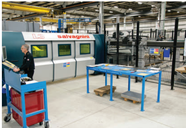
FIGURE 4. The cutting-edge laser cutting department at Modula's production facility in Lewiston, ME, includes a Salvagnini L3 fiber laser.
